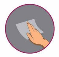
For fresh/new surfaces: Strip all loose particles from the surface with wire brushing and by scraping, followed by a wipe down. Wash the surface down with
